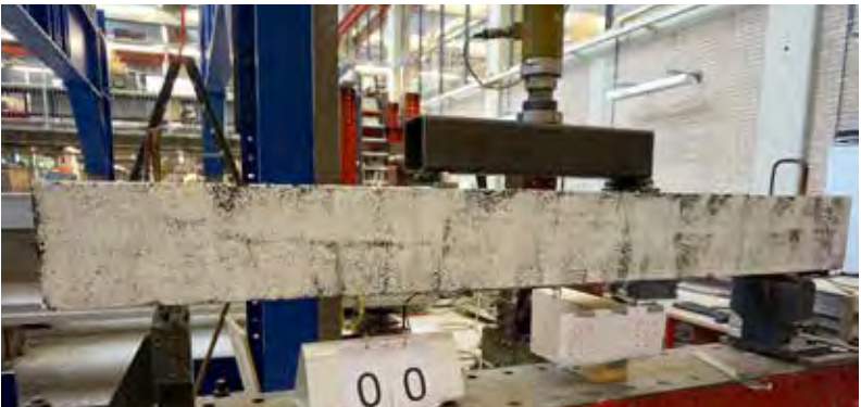
Fig 5 Test set-up. Left: painted side of beam for image analysis. Right: LVDTs to measure deformation.
