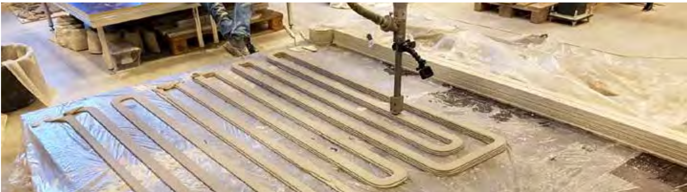
Fig. 3 Printing with one of the developed PVA-fiber reinforced Strain Hardening Cementitious Composites.
