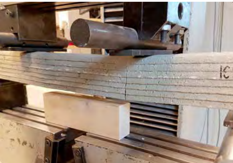
Fig. 6 Bending test on 3D printed concrete beam with cable reinforcement.
