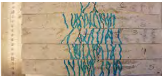
Fig. 3 Printing with one of the developed PVA-fiber reinforced Strain Hardening Cementitious Composites.
