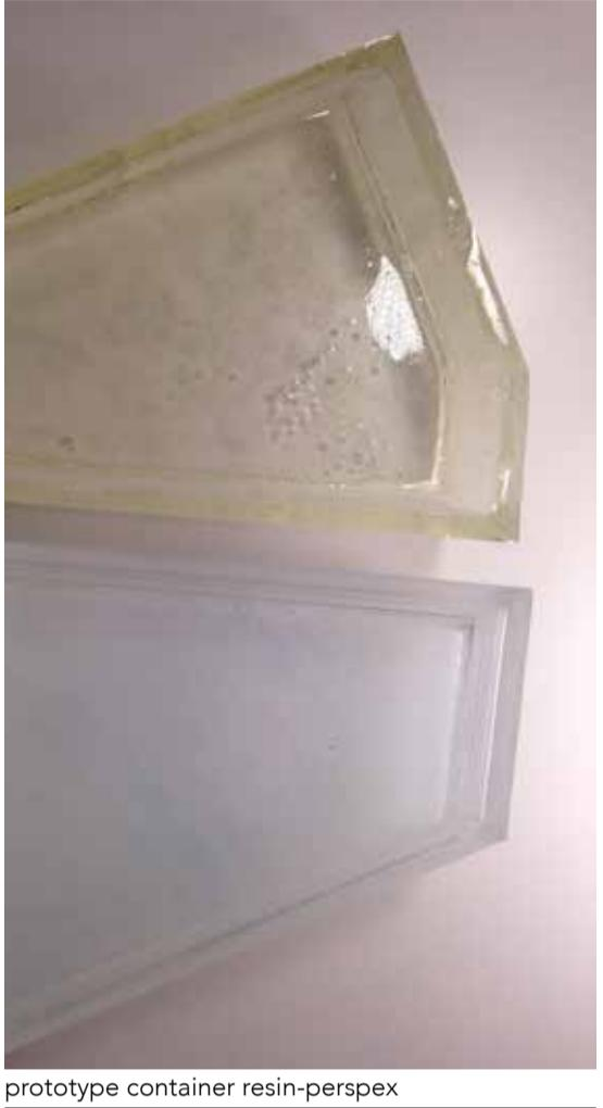
prototype container resin-perspex
