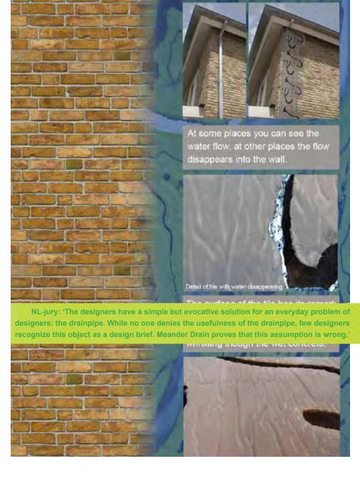
These tiles replace your drainpipe by meandering down the rain water.
