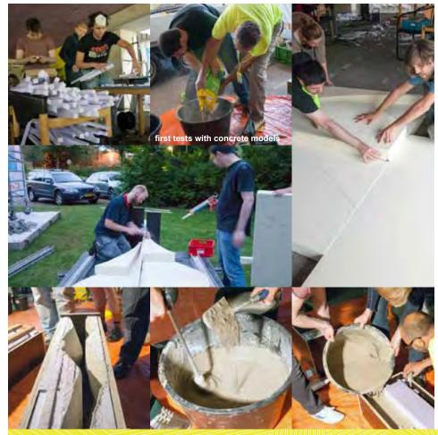
The prepared outside mould for the 1:1 prototype needed to be complemented with a foam core, determining the actual form of the object. Thinking, drawing, cutting, glueing and lots of sanding. Meanwhile the other groups produced their first concrete prototypes.
