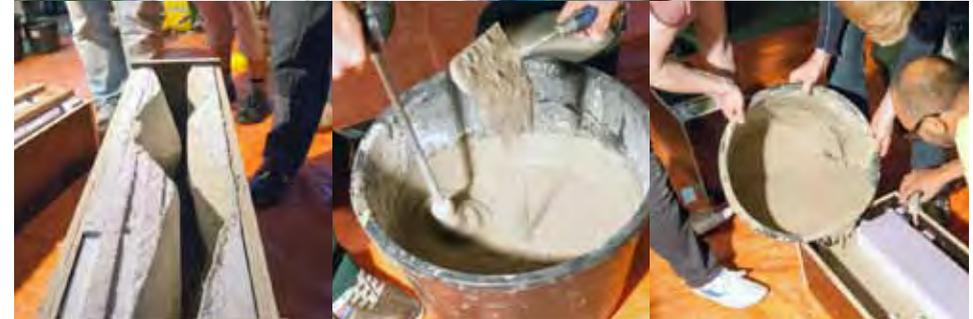
The prepared outside mould for the 1:1 prototype needed to be complemented with a foam core, determining the actual form of the object. Thinking, drawing, cutting, glueing and lots of sanding. Meanwhile the other groups produced their first concrete prototypes.
